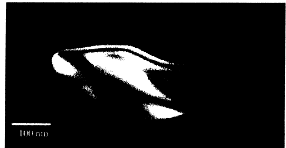
Fig. 3. Transmission electron microscopy picture of Si-grain after 1 h of oxidation at 1000^\circ\text{C} . The \text{SiO}_2 thickness around the silicon core corresponds to approximately 80 nm. Evidence of crystallinity of the entire grain core is manifested by diffraction fringes in bright field/dark field method. The surrounding \text{SiO}_2 is amorphous.
